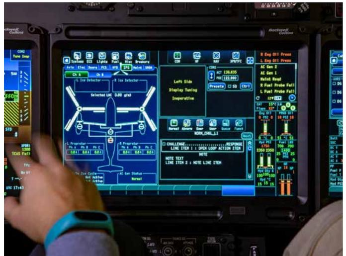
All eyes are on the sleek AW609 cockpit, made with real Pro-line Fusion Adaptive Flight Displays (AFDs), providing touchscreen monitors for aircraft interactive control and display functions. The AFDs give the aircrew the ability to interact not only with the primary flight, nacelle and navigation instrumentation, but also with the Flight Management System (FMS), aircraft synoptic, crew alert system, maps, charts and even more.
