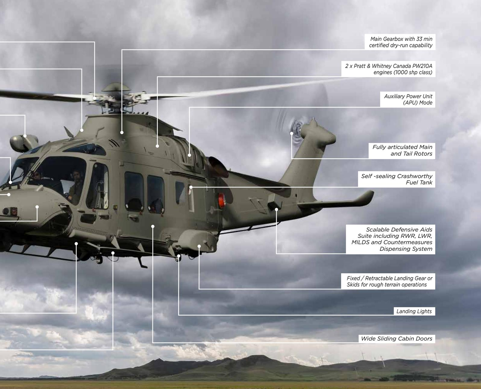
Main Gearbox with 33 min certified dry-run capability
