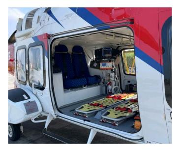
The AW169 features lifesaving equipment and two stretchers. The air ambulance is crewed by two pilots and supported by trained paramedics. The AW169 also provides night-time medevac capability to GVHL's client for their offshore facilities/operations.
