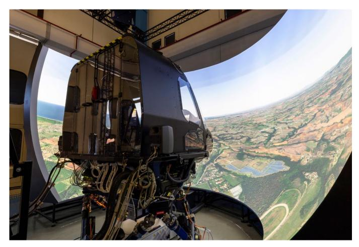
The unique Leonardo-developed simulator features go beyond compliance with FTD regulations and are instead more in line with Full Flight Simulator capabilities. The new ETD e-Motion incorporates a high-performance sixdegree-of-freedom motion system with short-throw six-inch actuators to realistically reproduce motion and vibration cues.
