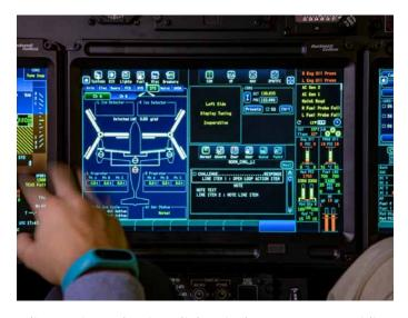
All eyes are on the sleek AW609 cockpit, made with real Pro-line Fusion Adaptive Flight Displays (AFDs), providing touchscreen monitors for aircraft interactive control and display functions. The AFDs give the aircrew the ability to interact not only with the primary flight, nacelle and navigation instrumentation, but also with the Flight Management System (FMS), aircraft synoptic, crew alert system, maps, charts and even more.
