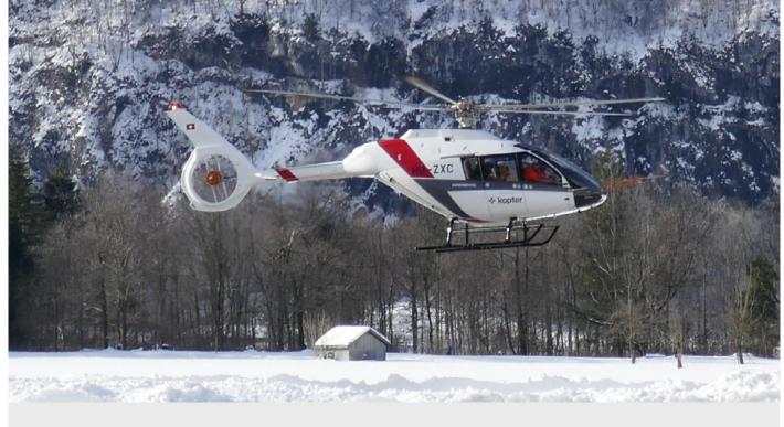
Since then, more than 40 flights have taken place and the crew has been able to expand the flight envelope to climb, descents, autorotation and turns up to 5,000ft.
