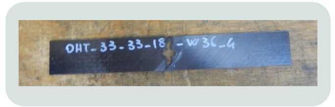
1-Open Hole Tension specimen after failure
